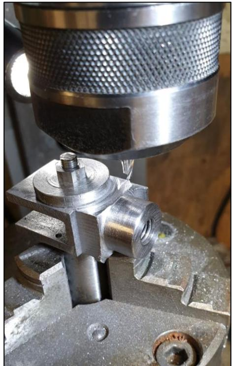
As can be seen here we have jumped a little, prior to this each blank was set in the 4 jaw and had its end boss turned and drilled/tapped 5/16 BSF.
