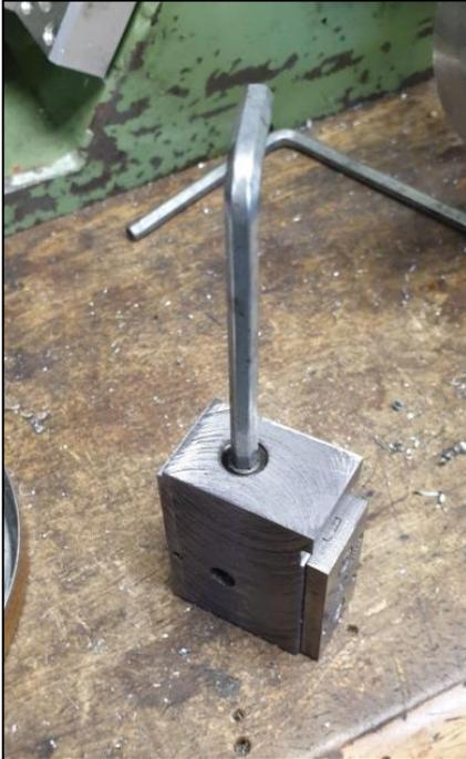
I have taken a different approach to make setting up a lot easier and less reliant on criticality. The piston rods are 5/16 stainless steel, I have threaded those 5/16 BSF and drilled/tapped the crossheads to match.
